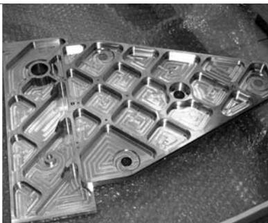
■ Finished rear surface. Differing wall thickness and pocket variations breaks up vibration
